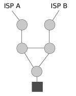
Provides a cheap form of multihoming with hostile ISPs. Motivated by the IETF Homenet working group. Works great with MP-TCP.
